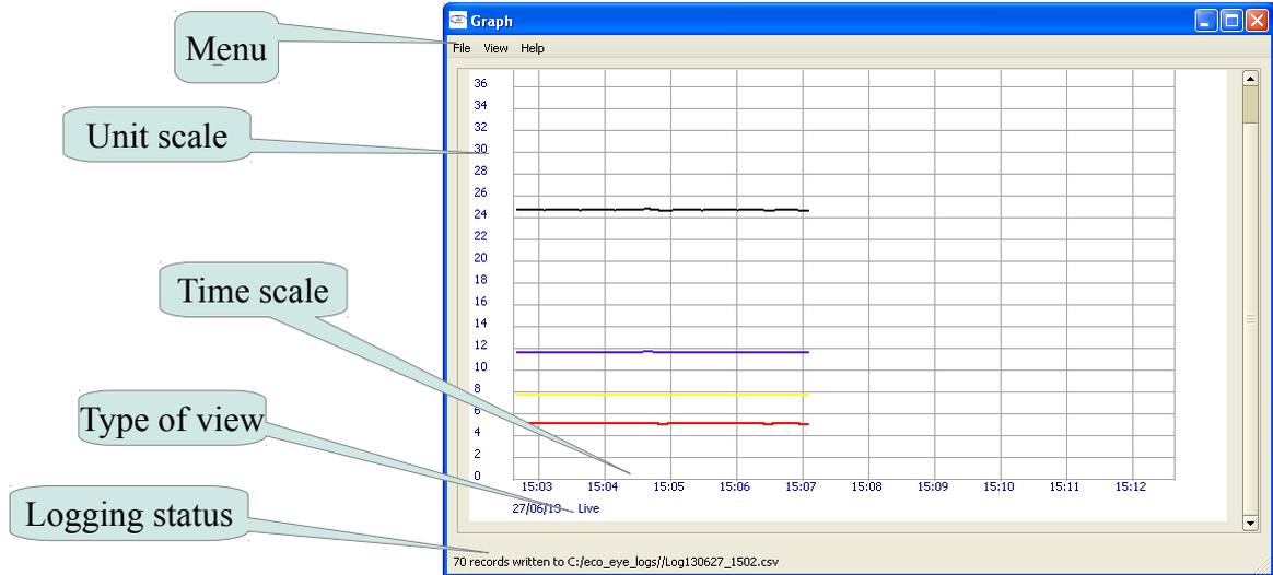
*The graph starts at the left and will scroll automatically when it reaches the right hand edge. The 3 phases are only shown in the Amps graph*
