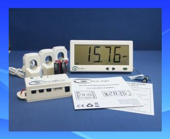
The Eco-eye Elite 200 electricity monitor can be used to identify wastage and help businesses to meet their energy efficiency targets - suitable for use in most commercial and industrial settings
